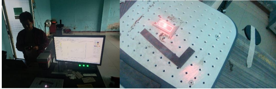
Figure 1. Laser Marking Process on SKD-11 Tool Steel
